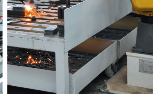
\pm 0.2 Open groove robot Steel laser cutting precision: \pm 0.2\text{mm}
