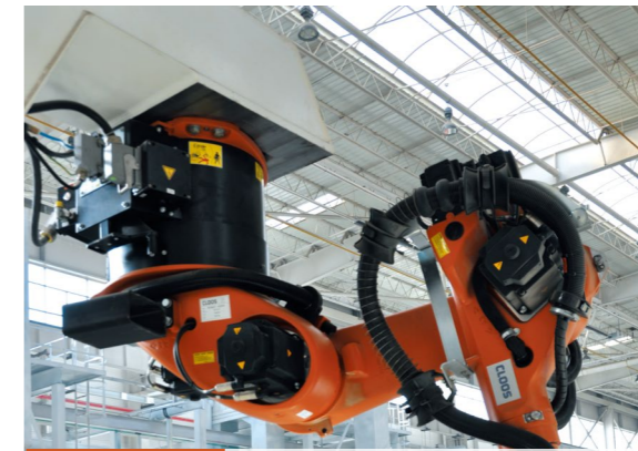
0.1 CLOOS robot Repositioning and flip precision reaches 0.1mm Arc automatic tracking system \leq 1\text{mm}
