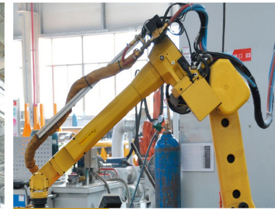
\pm 0.2 Open groove robot Steel laser cutting precision: \pm 0.2\text{mm}
