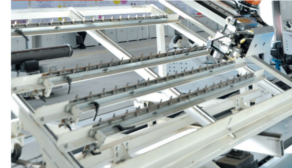
0.1 CLOOS robot Repositioning and flip precision reaches 0.1mm Arc automatic tracking system \leq 1\text{mm}
